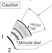
①Do not try to fold four setting pins next to the current time display(\*).you can not set these times. if you force it, you maby damage the switch.
