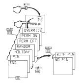
If a PIN code has been activated, the timer can no longer be activated without a valid PIN code after a RESET.
