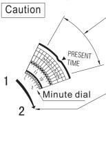
①Do not try to fold the four setting pins next to the current time display(\*).you can not set these times. if you force it, you maby damage the switch.
