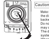
Make sure to turn the minute hand knob only in the direction shown by the arow. Turning it backward forcibly may damage the switch Do not try to turn the dial palte itself.you may cause a malfunction The dial shows the time using a 24 hour
